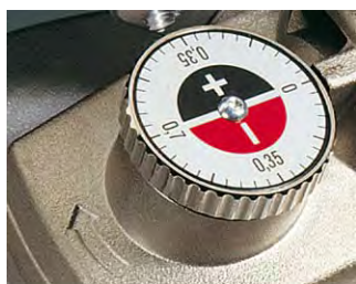
Adjustable milling height
