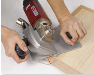
Flush-planing efficiently and clean
