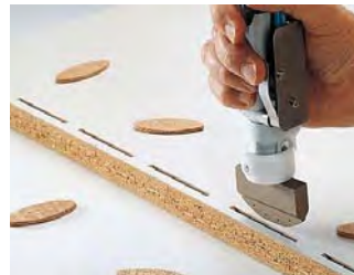
Nozzles for grooves
