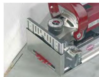
Cutting expansion gaps
