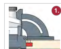
Cut groove 8 mm
