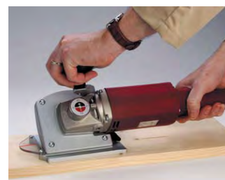
Planing protruding patch
