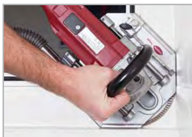
Deep cuts into the corner with the Tanga Delta S2
