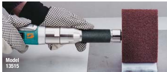
13515 Dynastraight® sets grain pattern in stainless steel.
