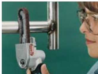
Clean and finish using non-woven nylon belts.
