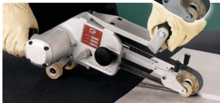
Place 11486 Dynabelter handle at 45° angle from belt housing to increase grinding pressure. Pull tool toward operator for faster material removal.
