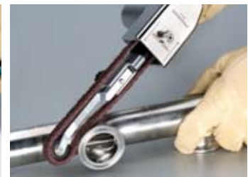
Clean and finish using non-woven nylon belts.
