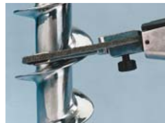
Clean and finish using non-woven nylon belts.
