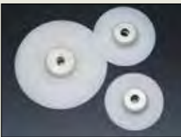
Flexible backing pads for using abrasive discs on angle sanders and grinders. 623279000 - 4 1/2" w/ M14-2.0 nut 623283000 - 4 1/2" w/ 5/8-11 nut 623284000 - 5" w/ 5/8-11 nut 623281000 - 7" w/ 5/8-11 nut 623282000 - 9" w/ 5/8-11 nut
