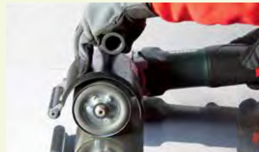
Preparation for mirror polishing: Metabo SE12-115 Burnisher with expansion roller, and Pyramid sanding belts from A160 (120 grit) to A6 (2000 grit).
