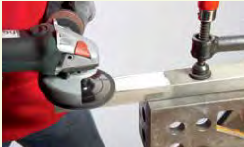
Preparation for Polishing; Metabo WE14-125 INOX 5" grinder, 5" 'cling fit' Pyramid sanding discs in grit range from A160 (120 grit) to A30 (600 grit) with 5" backing pad 623298000.
