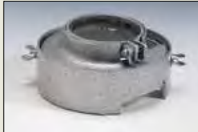
623276000 Cup wheel guard for mounting 3 1/8" Type 6 cup wheels on 4 1/2" - 6" angle grinders. Fits W7, W10 and prior WE14 series grinders.
