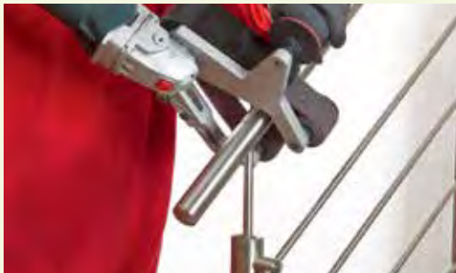
The RBE12-180 Pipe and Tube sander for a uniform even finish on hand rails using Pyramid sanding belts from A160 (120 grit) to A6 (2000 grit).
