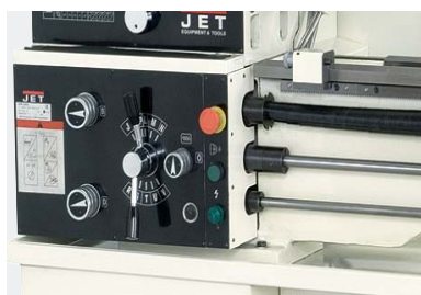
Gear box makes it possible to cut a number of threads without changing the gears
