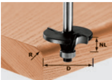
HW s = 8 Counterprofile cutter spring HW with ball bearing guide, shank 8 mm
