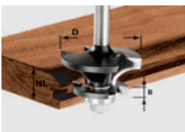
HW s = 8 Counterprofile cutter groove HW with ball bearing guide, shank 8 mm
