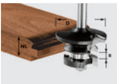
HW s = 8 Counterprofile cutter groove HW with ball bearing guide, shank 8 mm
