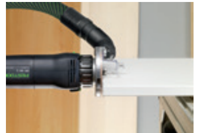
Rounding plastic or solid wood veneer.
