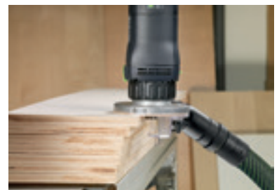
Chamfering plastic or solid wood veneer.
