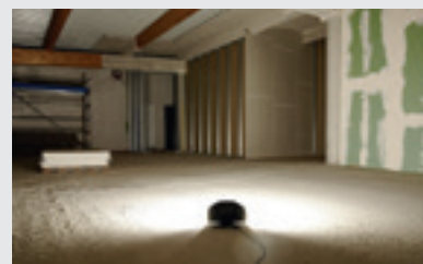
Festool SYSLITE DUO 180° scattering angle, uniform two-dimensional illumination, replicates the colour of daylight.
