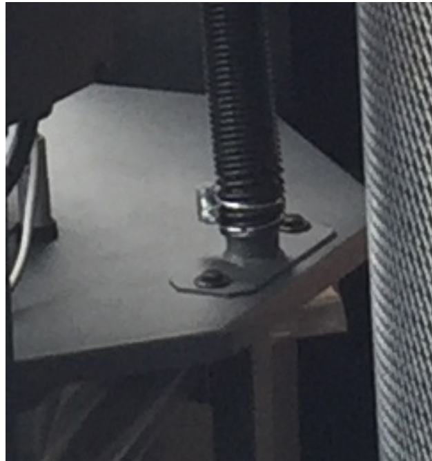
Drum lid vacuum suction tube
