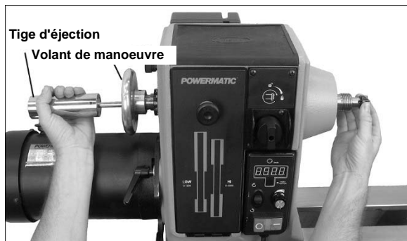
Figure 8-5 : Retirer la pointe
