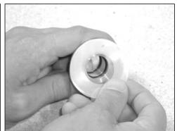
C. Attach the anti-friction ring.
